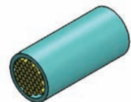
Duct containing 48 x Ø 1.2mm cable
